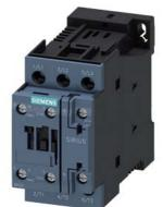
power contactor, AC-3e/AC-3, 17 A, 7.5 kW / 400 V, 3-pole, 72 V DC, auxiliary contacts: 1 NO + 1 NC, screw terminal, size: S0
