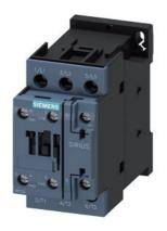
power contactor, AC-3e/AC-3, 17 A, 7.5 kW / 400 V, 3-pole, 42 V AC, 50/60 Hz, auxiliary contacts: 1 NO + 1 NC, screw terminal, size: S0, upright mounting position
