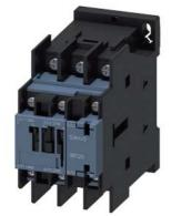
power contactor, AC-3e/AC-3, 12 A, 5.5 kW / 400 V, 3-pole, 400 V AC, 50 Hz / 400-440 V, 60 Hz, auxiliary contacts: 1 NO + 1 NC, ring cable lug connection, size: S0
