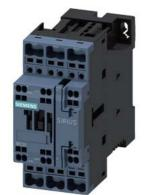
power contactor, AC-3e/AC-3, 12 A, 5.5 kW / 400 V, 3-pole, 95-130 V AC/DC, 50/60 Hz, with integrated varistor, auxiliary contacts: 1 NO + 1 NC, spring-loaded terminal, size: S0
