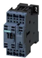
power contactor, AC-3e/AC-3, 12 A, 5.5 kW / 400 V, 3-pole, 24 V DC, 0.7-1.25\* Us, with plugged-in varistor, auxiliary contacts: 1 NO + 1 NC, spring-loaded terminal, size: S0, suitable for PLC outputs, not expandable with auxiliary switch
