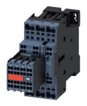
power contactor, AC-3e/AC-3, 12 A, 5.5 kW / 400 V, 3-pole, 24 V DC, with plugged-in diode combination, auxiliary contacts: 2 NO + 2 NC, spring-loaded terminal, size: S0, captive auxiliary switch
