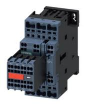
power contactor, AC-3e/AC-3, 12 A, 5.5 kW / 400 V, 3-pole, 230 V AC, 50/60 Hz, auxiliary contacts: 2 NO + 2 NC, spring-loaded terminal, size: S0, captive auxiliary switch, no surge suppressor retrofittable
