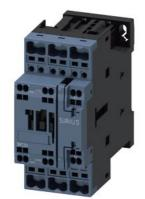
power contactor, AC-3e/AC-3, 12 A, 5.5 kW / 400 V, 3-pole, 24 V AC, 50 Hz, auxiliary contacts: 1 NO + 1 NC, spring-loaded terminal, size: S0, upright mounting position
