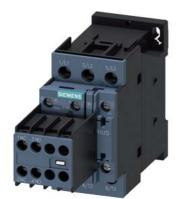
power contactor, AC-3e/AC-3, 12 A, 5.5 kW / 400 V, 3-pole, 220 V AC, 50/60 Hz, auxiliary contacts: 2 NO + 2 NC, screw terminal, size: S0, removable auxiliary switch
