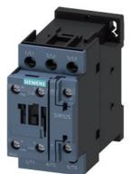
power contactor, AC-3e/AC-3, 12 A, 5.5 kW / 400 V, 3-pole, 100 V AC, 50 Hz / 100-110 V, 60 Hz, auxiliary contacts: 1 NO + 1 NC, screw terminal, size: S0
