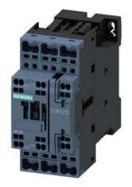
power contactor, AC-3e/AC-3, 9 A, 4 kW / 400 V, 3-pole, 220 V DC, auxiliary contacts: 1 NO + 1 NC, spring-loaded terminal, size: S0  $\,$
