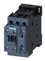
power contactor, AC-3e/AC-3, 9 A, 4 kW / 400 V, 3-pole, 24 V DC, 0.7-1.25\* Us, with plugged-in varistor, auxiliary contacts: 1 NO + 1 NC, screw terminal, size: S0, suitable for PLC outputs, not expandable with auxiliary switch
