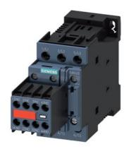
power contactor, AC-3e/AC-3, 9 A, 4 kW / 400 V, 3-pole, 24 V DC, with plugged-in diode combination, auxiliary contacts: 2 NO + 2 NC, screw terminal, size: S0, captive auxiliary switch
