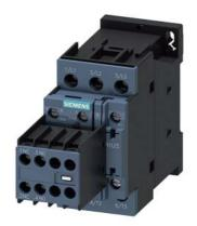
power contactor, AC-3e/AC-3, 9 A, 4 kW / 400 V, 3-pole, 24 V AC, 50 Hz, auxiliary contacts: 2 NO + 2 NC, screw terminal, size: S0, removable auxiliary switch
