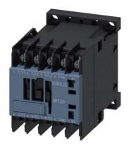
power contactor, AC-3e/AC-3, 16 A, 7.5 kW / 400 V, 3-pole, 200 V AC, 50 Hz / 200-220 V, 60 Hz, auxiliary contacts: 1 NC, ring cable lug connection, size: S00
