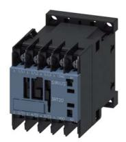
power contactor, AC-3e/AC-3, 16 A, 7.5 kW / 400 V, 3-pole, 200 V AC, 50 Hz / 200-220 V, 60 Hz, auxiliary contacts: 1 NO, ring cable lug connection, size: S00
