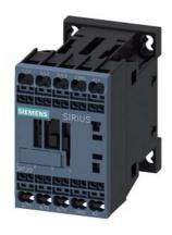
traction contactor, AC-3e/AC-3, 16 A, 7.5 kW / 400 V, 3-pole, 72-125 V DC, 0.7-1.25\* Us, electronic drive, with integrated varistor, auxiliary contacts: 1 NO, spring-loaded terminal, size: S00
