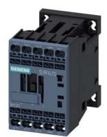
power contactor, AC-3e/AC-3, 16 A, 7.5 kW / 400 V, 3-pole, 24 V DC, with integrated diode, auxiliary contacts: 1 NO, spring-loaded terminal, size: S00  $\,$
