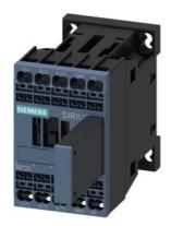
power contactor, AC-3e/AC-3, 16 A, 7.5 kW / 400 V, 3-pole, 110 V AC, 50 Hz / 120 V, 60 Hz, with plugged-on RC element, auxiliary contacts: 1 NO, spring-loaded terminal, size:  $\rm S00$
