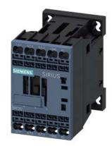
power contactor, AC-3e/AC-3, 16 A, 7.5 kW / 400 V, 3-pole, 230 V AC, 50/60 Hz, auxiliary contacts: 1 NO, spring-loaded terminal, size: S00
