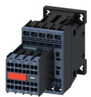
power contactor, AC-3e/AC-3, 16 A, 7.5 kW / 400 V, 3-pole, 110 V AC, 50 Hz / 120 V, 60 Hz, auxiliary contacts: 2 NO + 2 NC, spring-loaded terminal, size: S00, captive auxiliary switch
