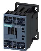
power contactor, AC-3e/AC-3, 16 A, 7.5 kW / 400 V, 3-pole, 110 V AC, 50 Hz / 120 V, 60 Hz, auxiliary contacts: 1 NC, spring-loaded terminal, size: S00  $\,$
