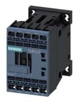
power contactor, AC-3e/AC-3, 16 A, 7.5 kW / 400 V, 3-pole, 42 V AC, 50/60 Hz, auxiliary contacts: 1 NO, spring-loaded terminal, size: S00
