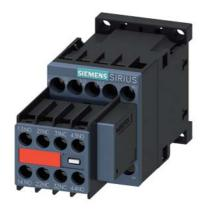
power contactor, AC-3e/AC-3, 16 A, 7.5 kW / 400 V, 3-pole, 230 V AC, 50/60 Hz, with varistor plugged on, auxiliary contacts: 2 NO + 2 NC, screw terminal, size: S00, captive auxiliary switch
