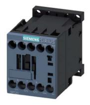
power contactor, AC-3e/AC-3, 16 A, 7.5 kW / 400 V, 3-pole, 12 V DC, auxiliary contacts: 1 NC, screw terminal, size: S00  $\,$
