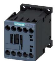
contactor, NEMA version, 5 HP, 460 / 575 V, 3-pole, 480 V AC, 60 Hz, auxiliary contacts: 1 NO, screw terminal, size: S00
