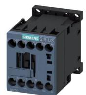
power contactor, AC-3e/AC-3, 16 A, 7.5 kW / 400 V, 3-pole, 380 V AC, 50/60 Hz, auxiliary contacts: 1 NC, screw terminal, size: S00  $\,$
