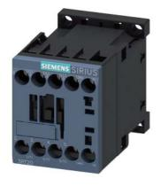
contactor, NEMA version, 5 HP, 460 / 575 V, 3-pole, 220 V AC, 50 Hz / 240 V, 60 Hz, auxiliary contacts: 1 NO, screw terminal, size: S00
