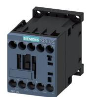
power contactor, AC-3e/AC-3, 16 A, 7.5 kW / 400 V, 3-pole, 100 V AC, 50 Hz / 100-110 V, 60 Hz, auxiliary contacts: 1 NC, screw terminal, size: S00
