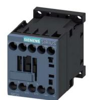
power contactor, AC-3e/AC-3, 16 A, 7.5 kW / 400 V, 3-pole, 42 V AC, 50/60 Hz, auxiliary contacts: 1 NO, screw terminal, size: S00
