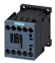
power contactor, AC-3e/AC-3, 16 A, 7.5 kW / 400 V, 3-pole, 24 V AC, 50/60 Hz, auxiliary contacts: 1 NO, screw terminal, size: S00  $\,$
