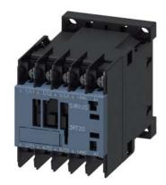
power contactor, AC-3e/AC-3, 12 A, 5.5 kW / 400 V, 3-pole, 400 V AC, 50 Hz / 400-440 V, 60 Hz, auxiliary contacts: 1 NO, ring cable lug connection, size: S00
