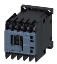
power contactor, AC-3e/AC-3, 12 A, 5.5 kW / 400 V, 3-pole, 110 V AC, 50 Hz / 120 V, 60 Hz, auxiliary contacts: 1 NO, ring cable lug connection, size: S00
