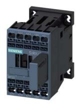
power contactor, AC-3e/AC-3, 12 A,  $5.5\,kW$  / 400 V, 3-pole, 24 V DC,  $0.85\text{-}1.85^*$  Us, with varistor plugged on, auxiliary contacts: 1 NO, spring-loaded terminal, size: S00, not expandable with auxiliary switch
