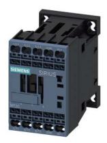
power contactor, AC-3e/AC-3, 12 A, 5.5 kW / 400 V, 3-pole, 24 V DC, 0.85-1.85  $^{\star}$  Us, with integrated diode, auxiliary contacts: 1 NC, spring-loaded terminal, size: S00, not expandable with auxiliary switch
