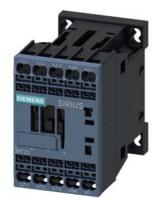
power contactor, AC-3e/AC-3, 12 A, 5.5 kW / 400 V, 3-pole, 24 V DC, 0.85-1.85\* Us, with integrated suppressor diode, auxiliary contacts: 1 NC, spring-loaded terminal, size: S00
