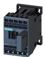
power contactor, AC-3e/AC-3, 12 A, 5.5 kW / 400 V, 3-pole, 24 V DC, 0.7-1.25\* Us, with varistor plugged on, auxiliary contacts: 1 NC, spring-loaded terminal, size: S00, not expandable with auxiliary switch
