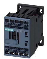
power contactor, AC-3e/AC-3, 12 A, 5.5 kW / 400 V, 3-pole, 24 V DC, 0.85-1.85\* Us, auxiliary contacts: 1 NO, spring-loaded terminal, size: S00, not expandable with auxiliary switch
