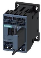
traction contactor, AC-3e/AC-3, 12 A, 5.5 kW / 400 V, 3-pole, 110 V DC, 0.7-1.25  $^{\star}$  Us, with integrated varistor, auxiliary contacts: 1 NC, spring-loaded terminal, size: S00, with plugged on series resistor
