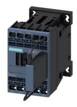
traction contactor, AC-3e/AC-3, 12 A, 5.5 kW / 400 V, 3-pole, 24 V DC, 0.7-1.25  $^{\star}$  Us, with integrated suppressor diode, auxiliary contacts: 1 NC, spring-loaded terminal, size: S00, with plugged on series resistor
