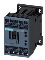
power contactor, AC-3e/AC-3, 12 A, 5.5 kW / 400 V, 3-pole, 48 V DC, with integrated diode, auxiliary contacts: 1 NC, spring-loaded terminal, size: S00  $\,$
