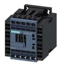
power contactor, AC-3e/AC-3, 12 A, 5.5 kW / 400 V, 3-pole, 110 V DC, with integrated diode, auxiliary contacts: 2 NO + 3 NC, spring-loaded terminal, size: S00, 3RH2921-2DA11 (1 NO + 1 NC), mounted left and right
