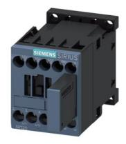
power contactor, AC-3e/AC-3, 12 A, 5.5 kW / 400 V, 3-pole, 24 V DC, 0.85-1.85  $^{\star}$  Us, with varistor plugged on, auxiliary contacts: 1 NO, screw terminal, size: S00, not expandable with auxiliary switch
