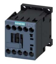
power contactor, AC-3e/AC-3, 12 A, 5.5 kW / 400 V, 3-pole, 24 V DC, 0.85-1.85  $^{\star}$  Us, with integrated diode, auxiliary contacts: 1 NO, screw terminal, size: S00, not expandable with auxiliary switch
