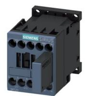
power contactor, AC-3e/AC-3, 12 A, 5.5 kW / 400 V, 3-pole, 24 V DC, 0.7-1.25\* Us, with varistor plugged on, auxiliary contacts: 1 NO, screw terminal, size: S00, not expandable with auxiliary switch
