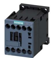
power contactor, AC-3e/AC-3, 12 A, 5.5 kW / 400 V, 3-pole, 24 V DC, 0.85-1.85\* Us, auxiliary contacts: 1 NC, screw terminal, size: S00, not expandable with auxiliary switch
