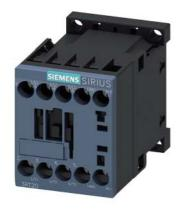
power contactor, AC-3e/AC-3, 12 A, 5.5 kW / 400 V, 3-pole, 24 V DC, 0.7-1.25\* Us, with integrated diode, auxiliary contacts: 1 NO, screw terminal, size: S00, suitable for PLC outputs, not expandable with auxiliary switch
