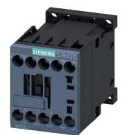
power contactor, AC-3e/AC-3, 12 A, 5.5 kW / 400 V, 3-pole, 48 V DC, auxiliary contacts: 1 NC, screw terminal, size: S00  $\,$
