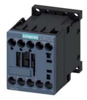
power contactor, AC-3e/AC-3, 12 A, 5.5 kW / 400 V, 3-pole, 24 V DC, auxiliary contacts: 1 NO, screw terminal, size: S00, communication-capable
