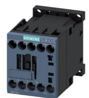
power contactor, AC-3e/AC-3, 12 A, 5.5 kW / 400 V, 3-pole, 600 V AC, 60 Hz, auxiliary contacts: 1 NC, screw terminal, size: S00
